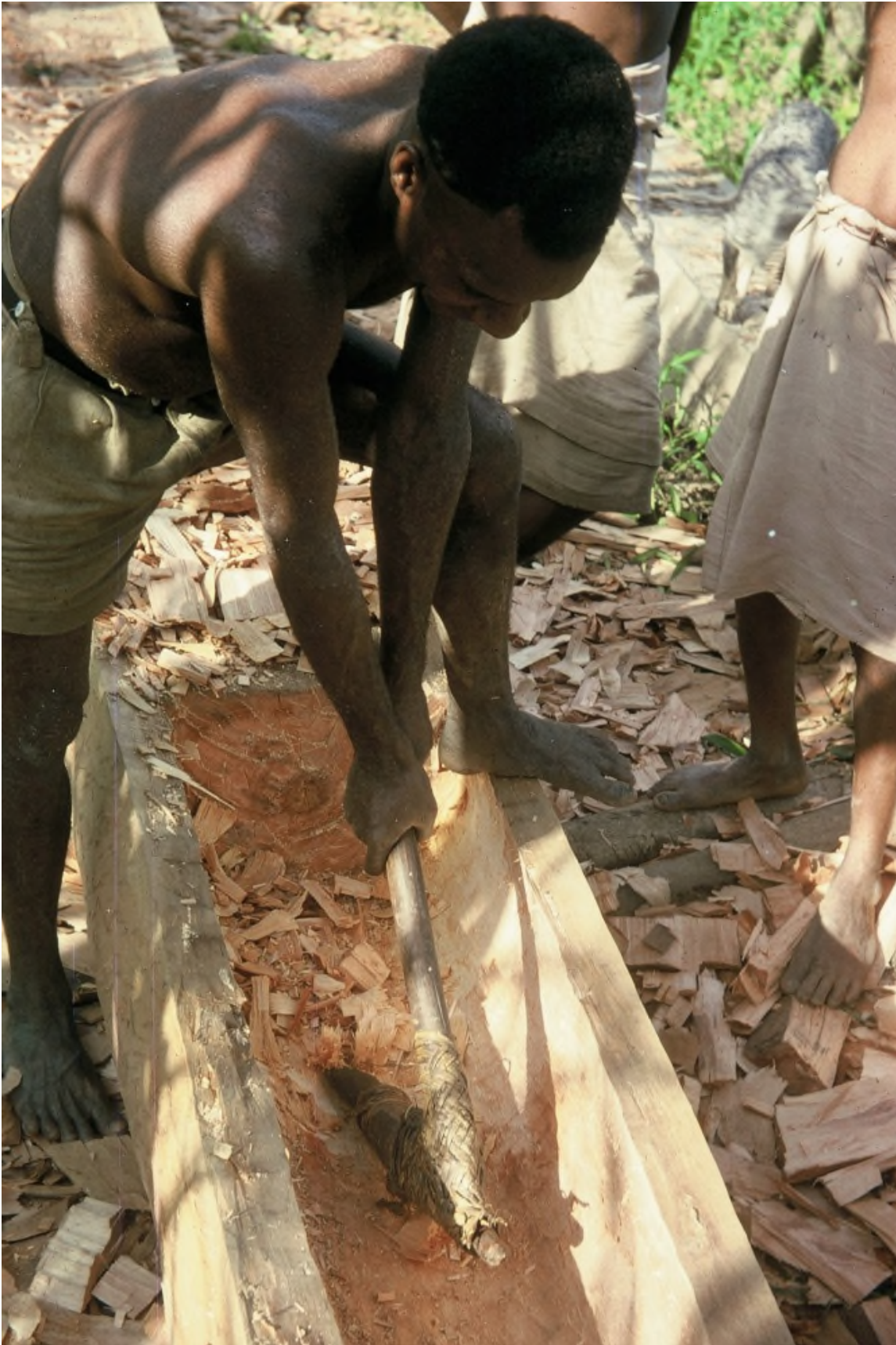
7. Man finishing off a canoe with a stone adze at a canoe making 'factory' (men like to work together and share the work over a number of canoes using a variety of tools). This man prefers a stone adze to finish off a canoe in order to give a firmer (smooth and crushed) surface to preserve the soft timber from water logging and rot. June 1967.
