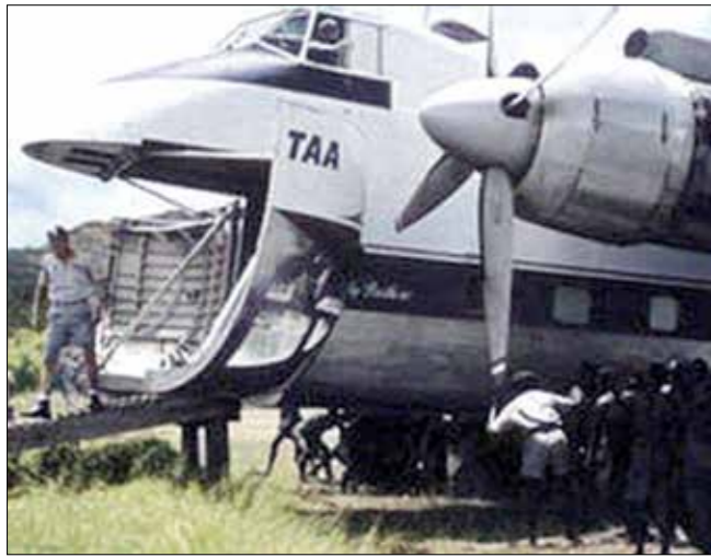
Moving B170 up to the ramp to unload a truck
